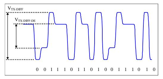
Figure 51. Differential transmitter post-cursor de-emphasized waveform
