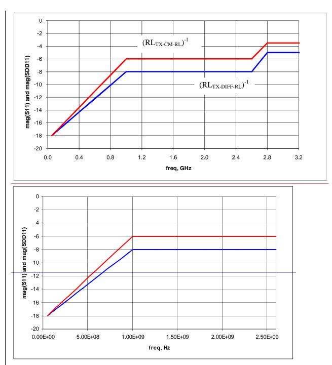
Figure 50. Transmit return loss mask
