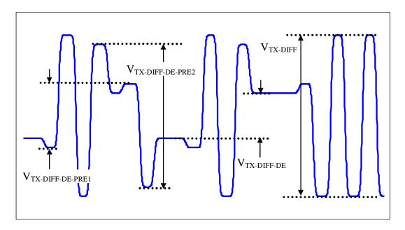
Figure 52. Transmit with pre- and post-cursor de-emphasis
