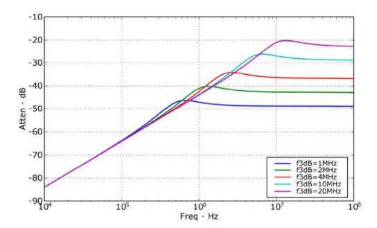
Figure 49. System reference clock jitter rejection
