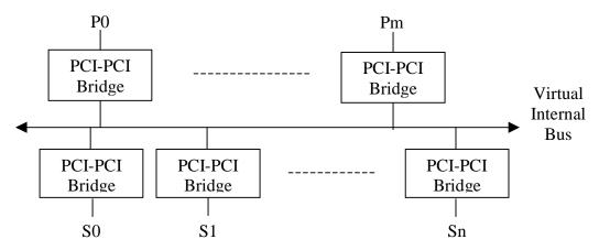
Figure 29. Logical Model of a Switch
