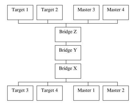
Figure 26. Example PCI System
