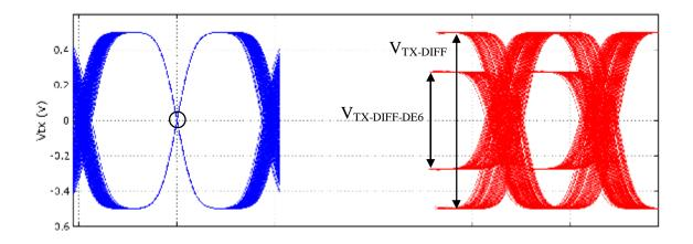
Figure 55. CLK to CAD data eye with some transmit jitter
