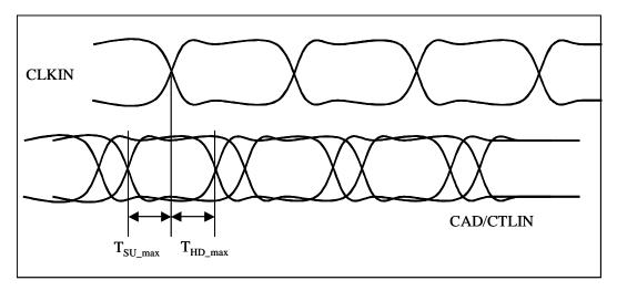
Figure 46.  $T_{SU}$  and  $T_{HD}$
