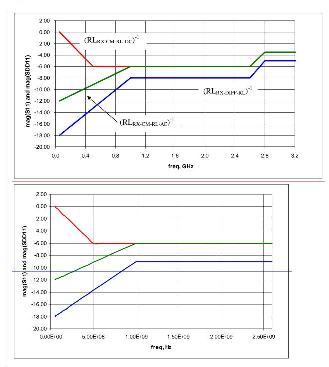
Figure 58. Receiver return loss mask
