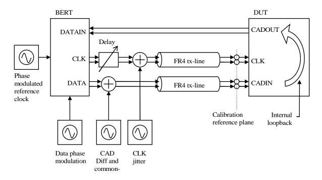
Figure 63. Receiver input compliance test setup
