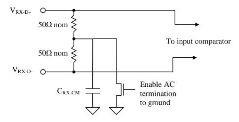
Figure 59. Receiver input termination
