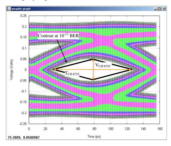
Figure 57. Channel compliance eye diagram
