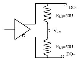
Figure 31. DC Output Reference System Load
