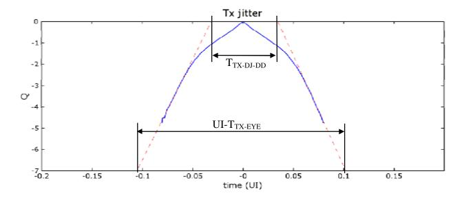
Figure 64. Transmit CAD jitter plotted on Q axis
