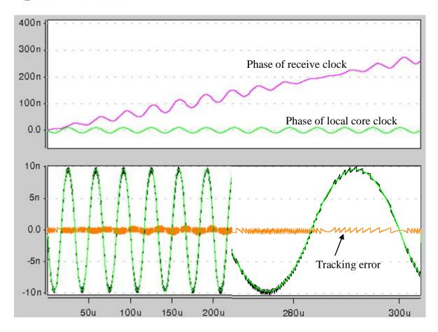
Figure 65. Phase tracking across receiver sync-fifo
