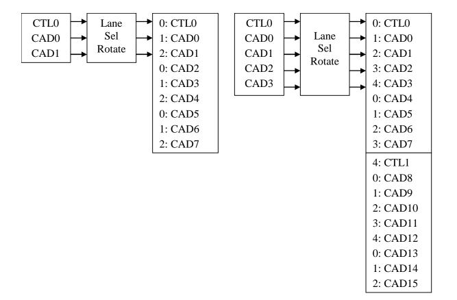
Figure 9. ILM Lane Mapping for Wide Transmitters
