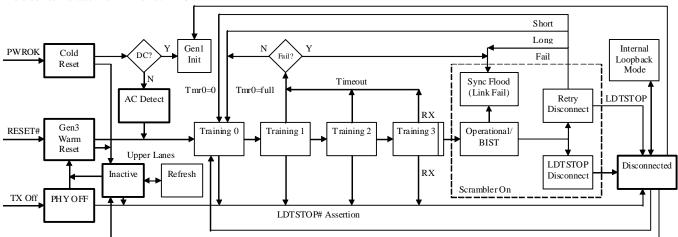
Figure 17. Link State Diagram
