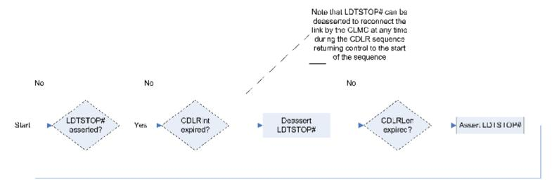
Figure 13. CLMC Sequencing Diagram for CDLR
