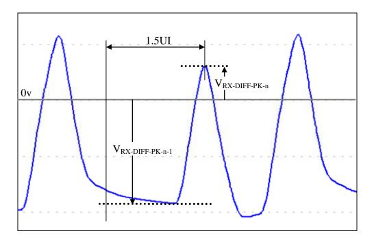
Figure 61. Receiver adjacent bit ratio
