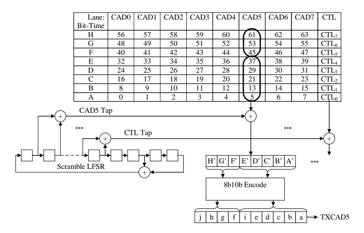
Figure 4. Gen3 Transmitter Order of Operations
