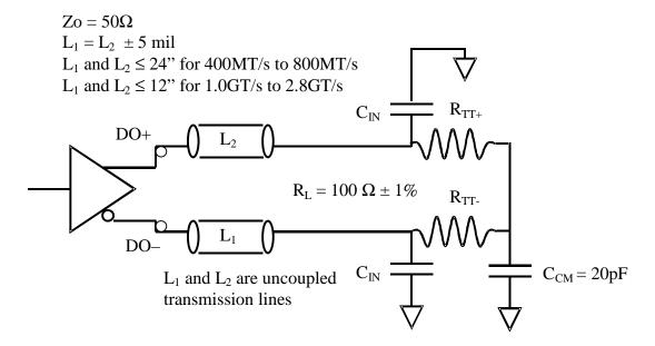
Figure 37. AC Reference System Load (See Table 168 for C<sub>IN</sub>, R<sub>TT+</sub> and R<sub>TT</sub>)
